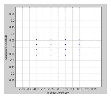
Observe that the scatter plot is stretched horizontally and compressed vertically compared to the undistorted constellation.
