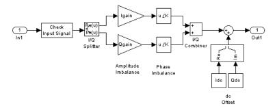
The value of the **I/Q amplitude imbalance (dB)** parameter is divided between the in-phase and quadrature components:
