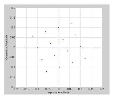
Observe that each point in the constellation is rotated by a 20 degree angle counterclockwise.
