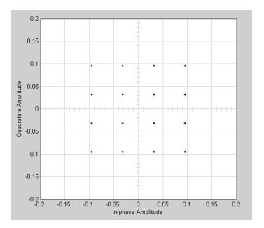
The following figure shows a scatter plot of an output signal, modulated by 16-ary QAM, from the I/Q block with **I/Q amplitude imbalance** (**dB**) set to 8 and all other parameters set to 0:
