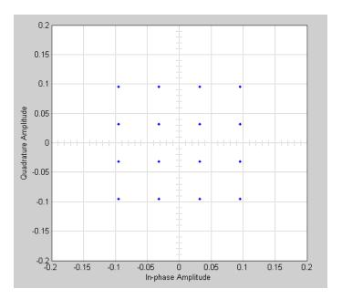
The following figure shows a scatter plot of an output signal, modulated by 16-ary QAM, from the Phase Noise block with **Phase noise level** (dBc/Hz) set to -70 and **Frequency offset** (Hz) set to 100:
