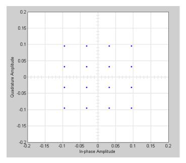
You can generate a scatter plot of the same signal after it passes through the Memoryless Nonlinearity block, with the **Method** parameter set to Saleh Model, as shown in the following figure.
