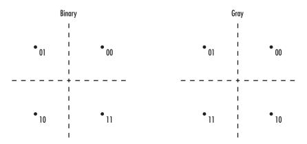
The figure below shows the signal constellation for the DQPSK modulation method when the **Phase rotation** parameter is  $\pi/4$ . The arrows indicate the four possible transitions from each symbol to the next symbol. The Binary and Gray options determine which transition is associated with each pair of input values.
