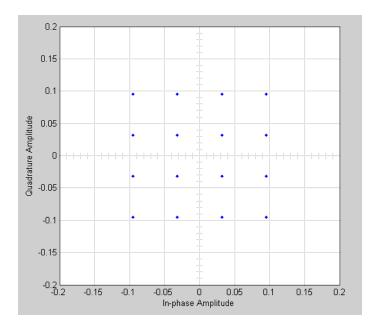
The following figure shows a scatter plot of an output signal, modulated by 16-ary QAM, from the Phase/Frequency Offset block with **Phase offset (deg)** set to 20 and **Frequency offset (Hz)** set to 0:
