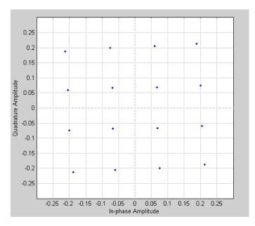
This plot is generated by the model described in "Scatter Plot Examples" with the following parameter settings for the Rectangular QAM Modulator Baseband block:
