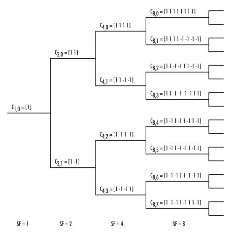
If [C] is a code length  $2^r$  at depth r in the tree, where the root has depth 0, the two branches leading out of C are labeled by the sequences  $[C\ C]$  and  $[C\ -C]$ , which have length  $2^{r+1}$ . The codes at depth r in the tree are the rows of the matrix  $C_N$ , where  $N=2^r$ .
