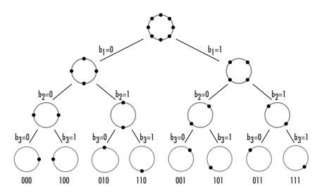
For other examples of signal constellations in set-partitioned order, see [1] or the reference pages for the M-PSK TCM Encoder and Rectangular QAM TCM Encoder blocks.
