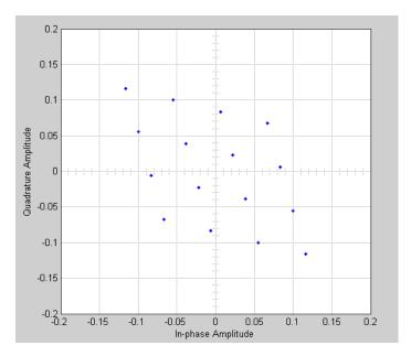
Setting the I dc offset to 0.02 and the  $\bf Q$  dc offset to 0.04 shifts the constellation 0.02 to the right and 0.04 up, as shown below:
