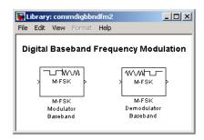
M-FSK Demodulator Baseband M-FSK Modulator Baseband Demodulate FSK-modulated data Modulate using M-ary frequency shift keying method
